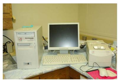
**33. Instrument Name:** Microcalorimeter
