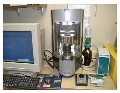
**45. Instrument Name:** Surface Tension Meter
