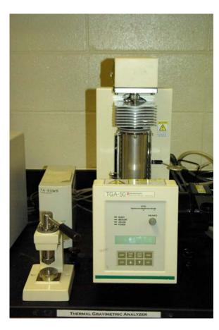
**46. Instrument Name:** Thermogravimetric Analyzer
