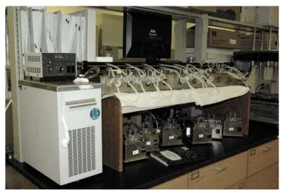
**41. Instrument Name:** Side-By-Side Diffusion Chambers
