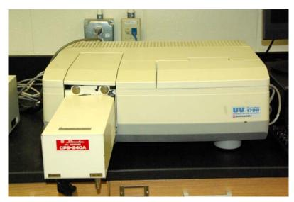
**55. Instrument Name:** UV/Visible Spectrophotometer
