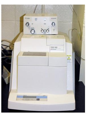
**14. Instrument Name:** Differential Scanning Calorimeter
