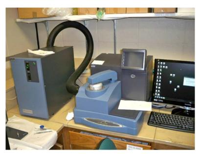
**32. Instrument Name:** Modulated Differential Scanning Calorimeter
