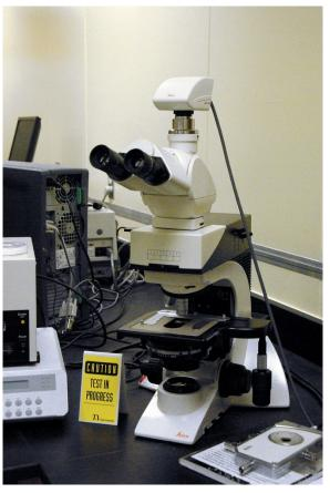
**16. Instrument Name:** Fluorescent Hot/cold stage polarized Microscope
